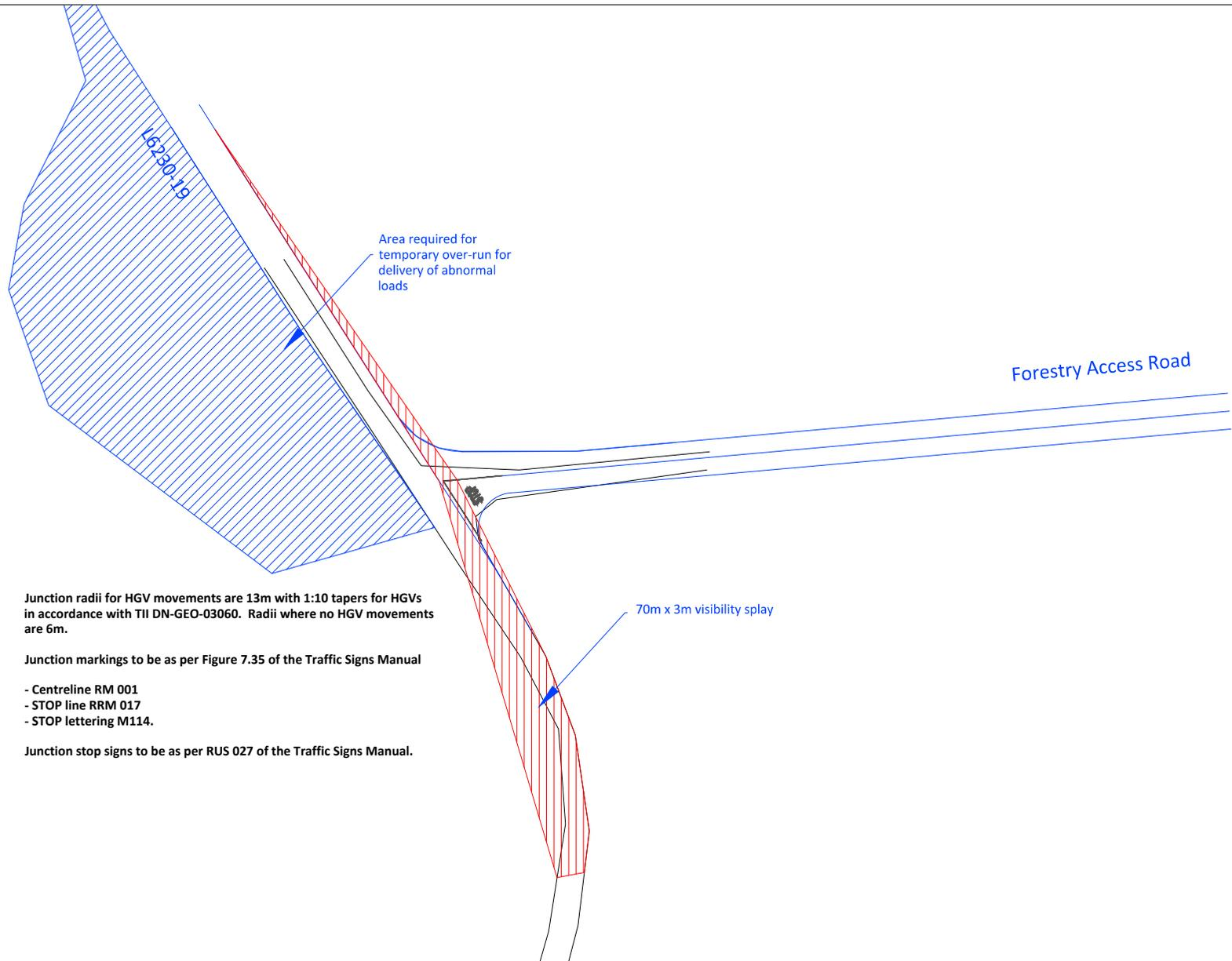
Junction radii for HGV movements are 13m with 1:10 tapers for HGVs in accordance with TII DN-GEO-03060. Radii where no HGV movements are 6m.
