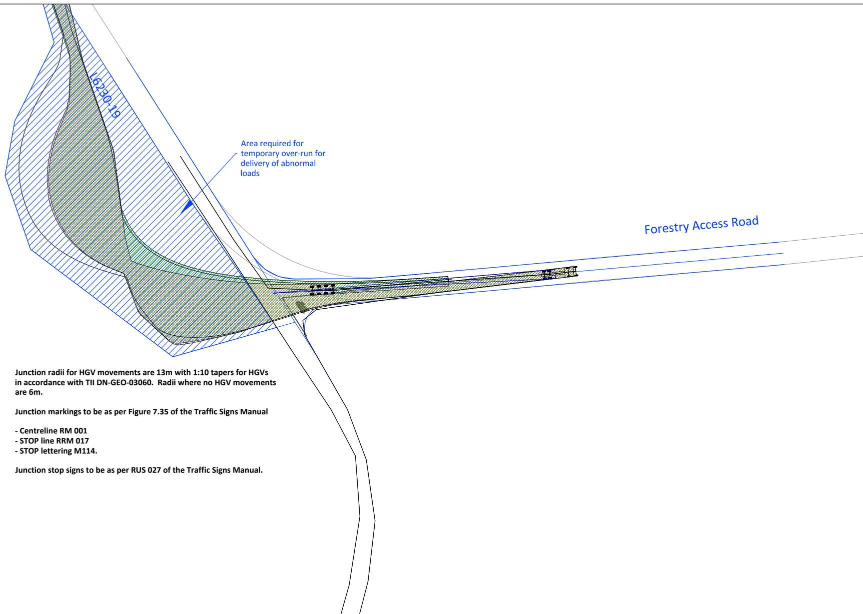
Junction radii for HGV movements are 13m with 1:10 tapers for HGVs in accordance with TII DN-GEO-03060. Radii where no HGV movements are 6m.
